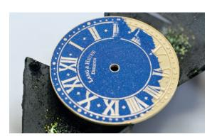
Hand-applied glass crystals fill the relief structure
